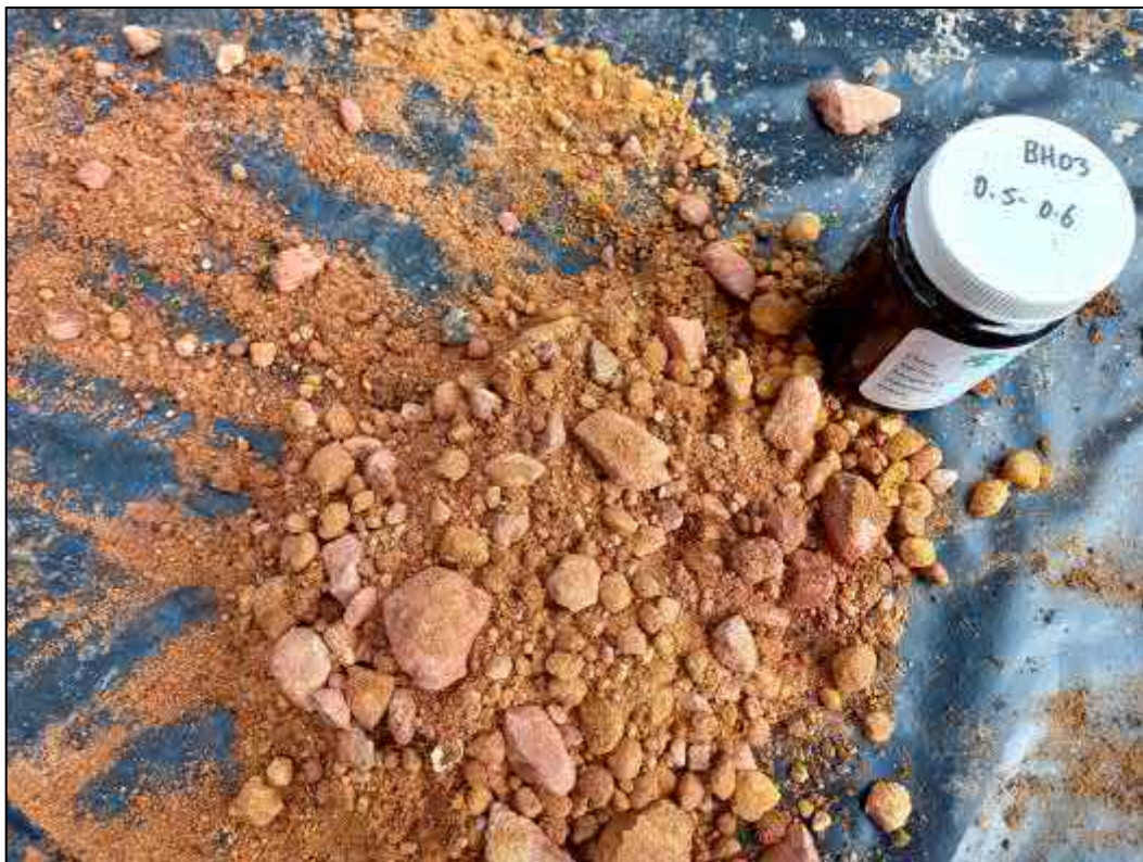
Photograph 6: Bore hole BH03. Weathered, medium grained, red and pale grey sandstone encountered from 0.5 m BGL.
