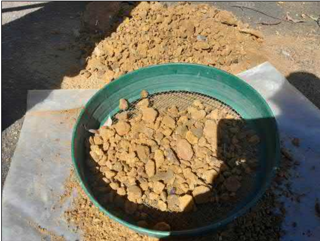
Photograph 15: Asbestos assessment included field screening of 10 Litre samples at all test pit locations.
