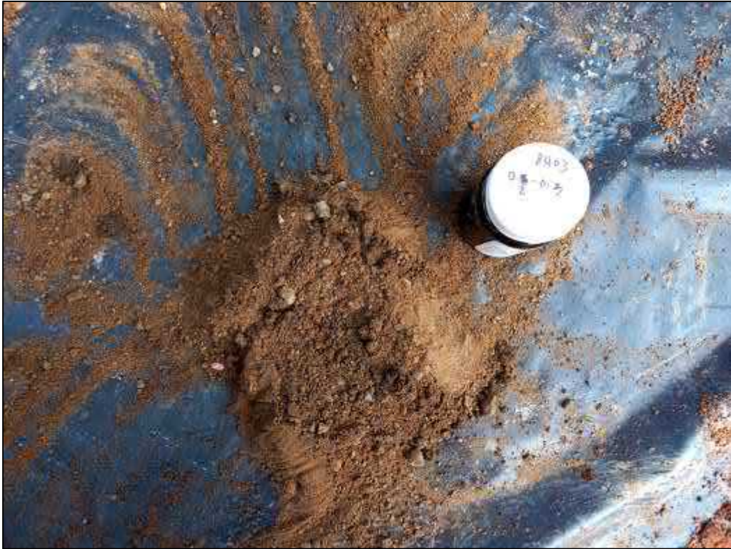
Photograph 5: Bore hole BH03 - Road base material consisting of mixed small to large angular gravels combined with coarse sand.
