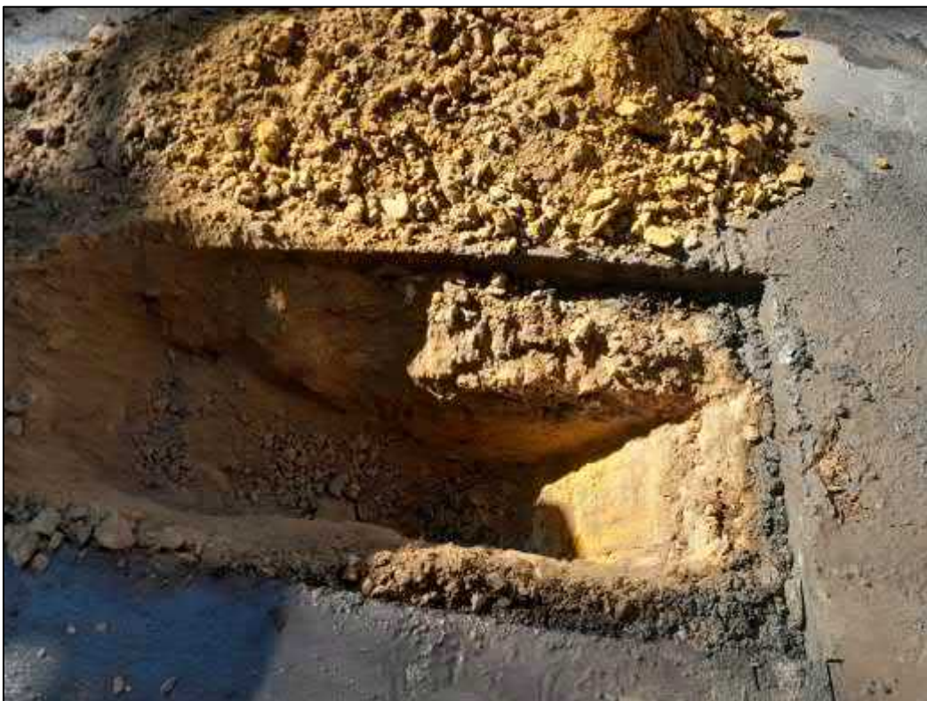
Photograph 12: Location TP02 with asphalt overlaying shallow fill (gravelly sand) with sand at 0.15 mBGL and natural sandy clay encountered from 0.3 mBGL (TP02)
