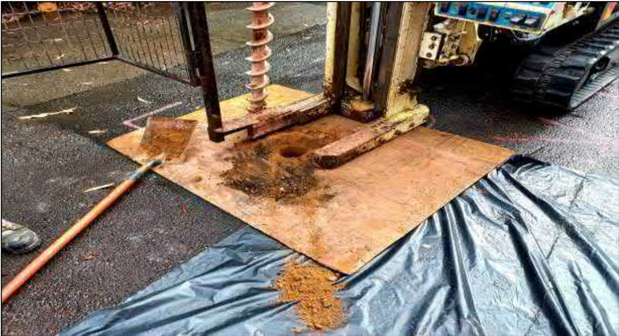
Photograph 3: Borehole BH02. Natural residual soil consisting of brown to red clayey sand material encountered from 0.3 m BGL.
