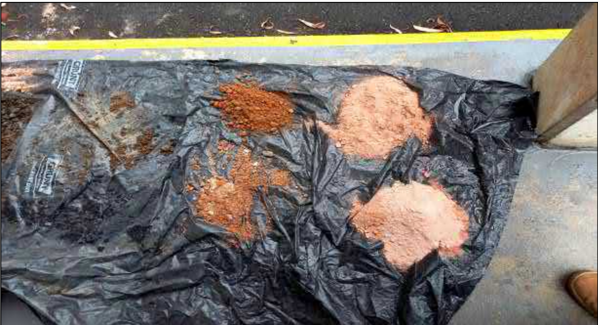
Photograph 4: Soil lithologies of fill and natural (left side) alongside bedrock material shown as pink highly weathered sandstone.
