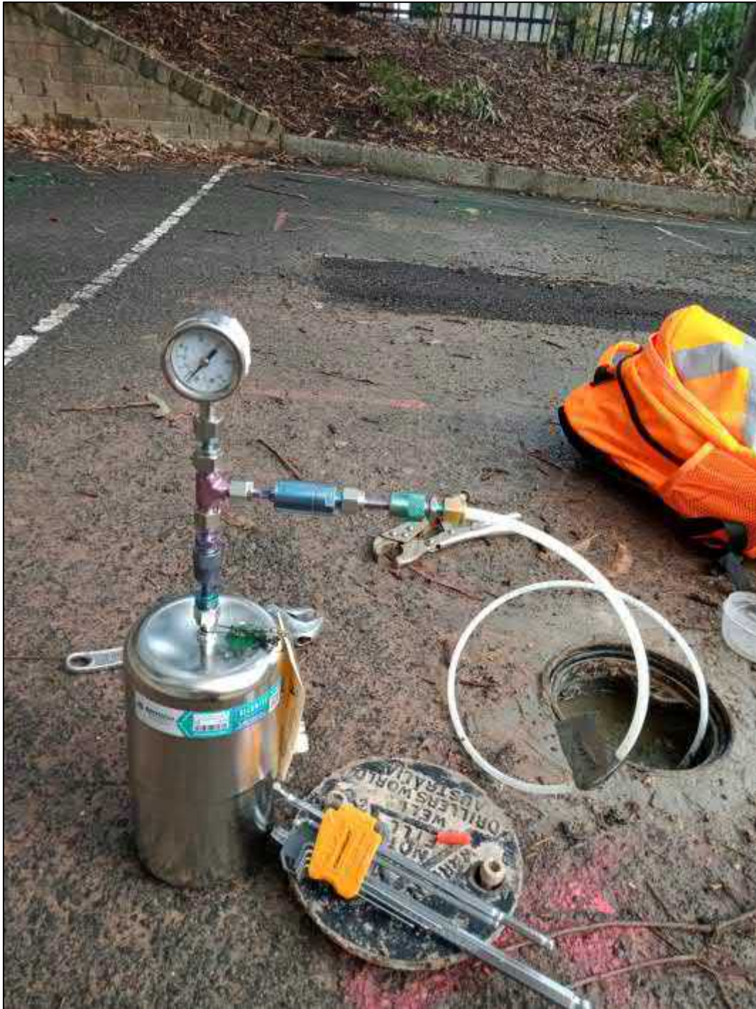
Photograph 17: Soil vapour sampling set-up.
