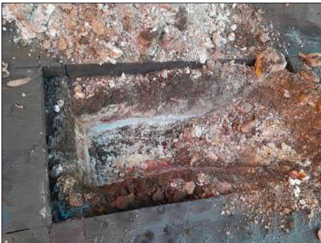
Photograph 14: Refusal on sandstone at 0.4 mBGL (TP05)
